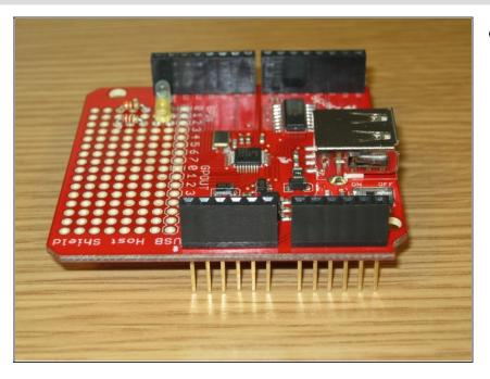
Solder stackable header pins to the USB Shield so that you can connect it to the Arduino and still be able to connect the XKitz boards on top. The order in which you finally stack the boards does not matter. Use blue-tack (again!) to keep the headers square while you flip over the board and solder the pins on the base of the board.
